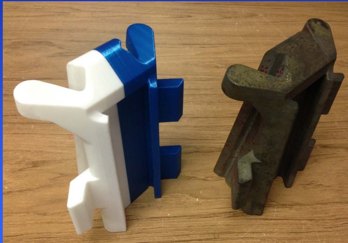
3D Printed 150K slip bowl carrier used to direct investment cast the carrier prototypes. 3D printing reduced the lead time to product testing by 3 months.
